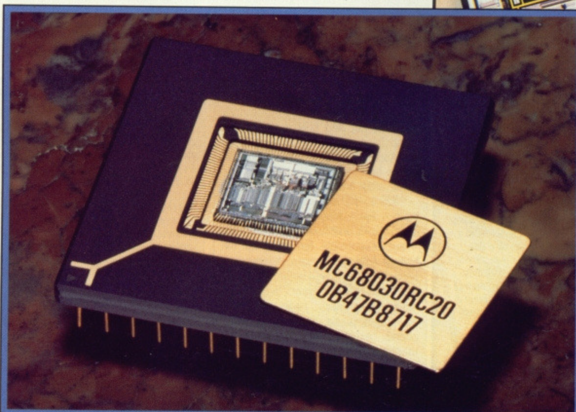
■ Motorola's 68030 microprocessor; the most recent member of the 68K family. "Oh-Thirty" is often described as a mainframe on a chip. The processor boasts a clock rate of 25MHz, instruction and data caches, parallel processing facilities, Burst Fill (a method of speeding up information transmission from memory) and 68K series compatibility. £300 if you want one!
