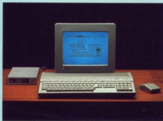
■ Modems: the Tandata TM500, on the left, with Microlink's intelligent modem next to it. On a manual modem you have to set the speed from a panel on the front, plug a telephone in the back and dial by hand. Intelligent modems are controlled directly by your computer.
