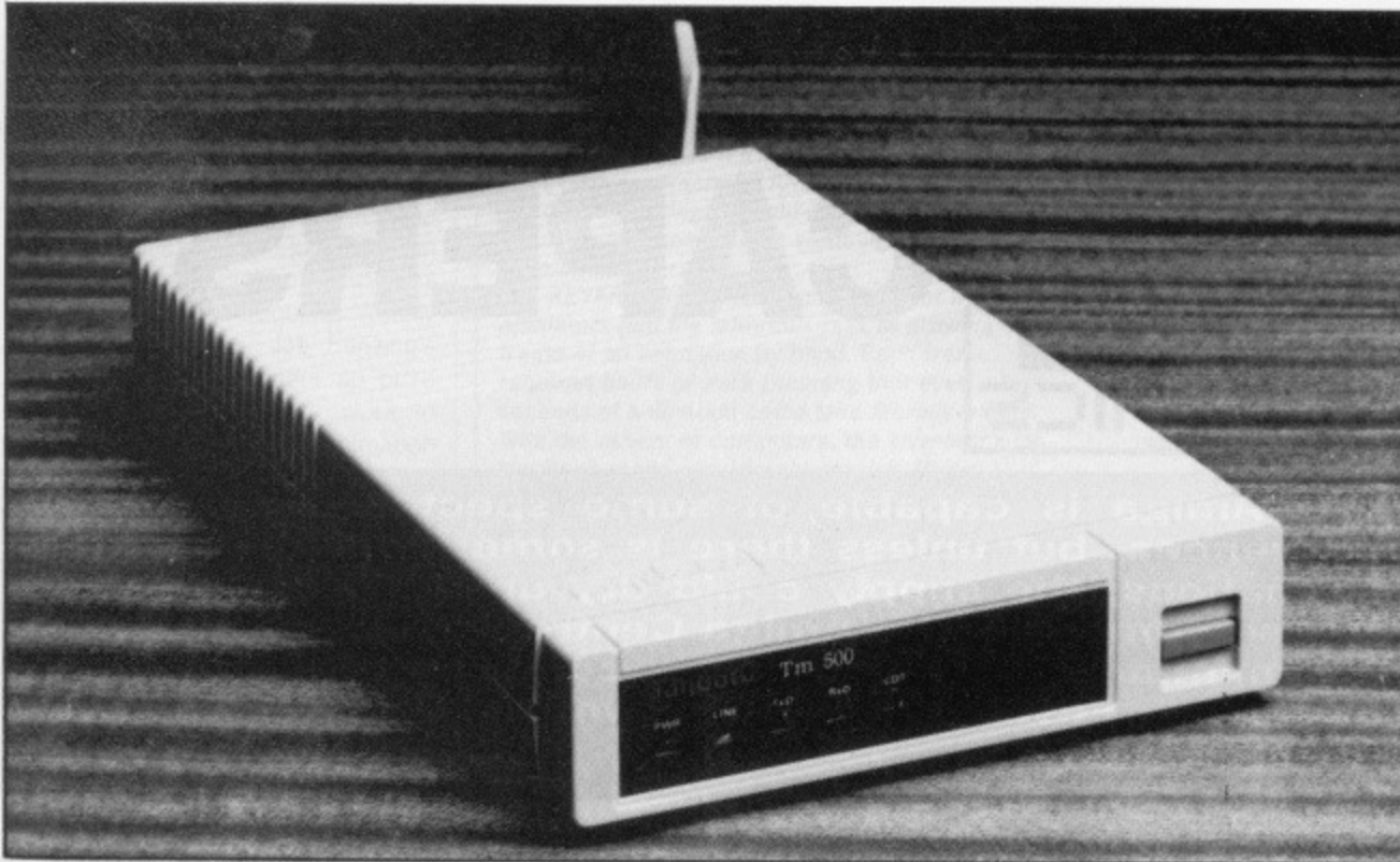
■ Tandata's Tm 500 is a very intelligent modem. Well, it must be; it doesn't have any buttons. The Tm500 offers auto-dial, Hayes compatibility, V21 300/300, V23 1200/1200, 1200/75 and 75/1200 - and all for £171.35.
